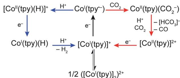
Scheme 3 Proposed mechanisms for CO<sub>2</sub> and H<sup>+</sup> reduction by Co-tpy.
