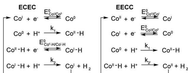
Scheme 2 ECEC and EECC schematic mechanisms for H<sub>2</sub> evolution by 1–5.
