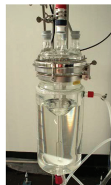
Fig. 11 \text{MgF}_2 sol stabilised by \text{Al}(\text{O}^i\text{Pr})_3 after 2 days of fluorination prepared in a 10 L reactor.
