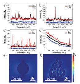
Fig. 2 SERS spectra of (a) R6G (5  $\times$  10  $^{-9}$  M), (b) 4-NBT (5  $\times$  10  $^{-8}$  M), (c) CV  $(1 \times 10^{-10} \text{ M})$ , and (d) NB  $(5 \times 10^{-11} \text{ M})$  obtained with a 632.8 nm excitation (2 mW, integration time = 10 s). FDTD-simulated |E| distributions of an (e) AuNP and (f) AuNPC.
