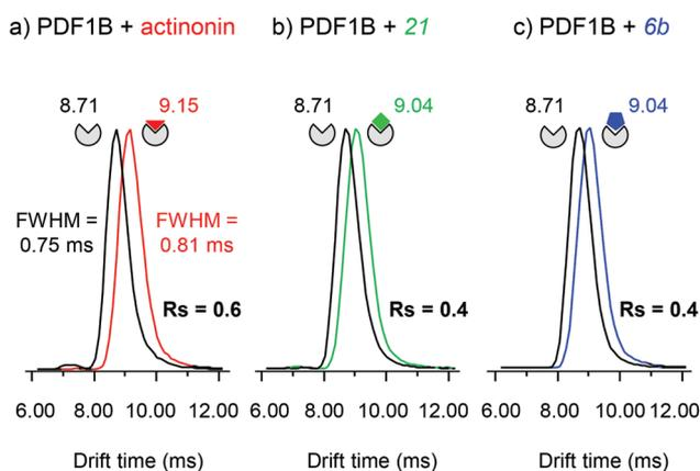
**Fig. 5** Ion-mobility mass spectrometry characterization of the conformational changes induced upon ligand binding on PDF1B. Extracted arrival drift time distributions (ATDs) of the 9+ charge states of PDF1B in the presence of sub-stoichiometric (1:0.5) (a) actinonin, (b) compound **21**, and (c) compound **6b** after 10 min incubation. The ATDs corresponding to PDF1B, PDF1B:actinonin, PDF1B:**21** and PDF1B:**6b** are shown in black, red, green and blue, respectively.
