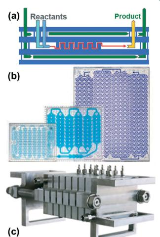
Fig. 5 Examples of commercial flow reactor systems for production. (a, b) Corning Advanced Flow Reactors (AFR);<sup>24</sup> (b) glass reactor plates of increasing size. Note the size of the static mixer structures remain similar with scaling of the plates. (Corning) (c) Lonza flow plate technology<sup>25</sup> in stainless steel. (Ehrfeld Mikrotechnik-BST).
