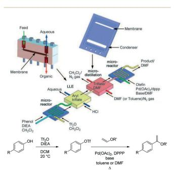
Fig. 6 Multistep reaction sequence with liquid-liquid extraction and single stage distillation for solvent switch.<sup>30</sup>
