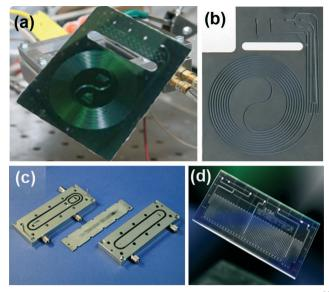
Fig. 3 Examples of microstructured reactors in (a) silicon-Pyrex, 20 (b) ceramics, <sup>21</sup> (c) stainless steel (IMM), <sup>16</sup> and (d) glass (Chemtrix). <sup>22</sup>
