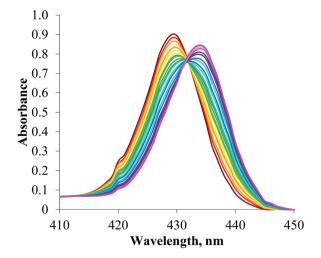
**Fig. 5** Changes in the Soret band of the UV/visible spectrum of a 2  $\mu$ m solution of porphyrin **5** upon addition of TBA-Cl (CHCl<sub>3</sub>, 293 K).
