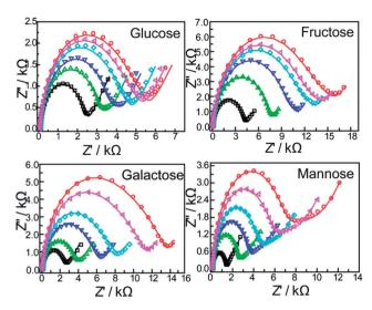
**Fig. 4** EIS of the modified gold electrodes modified with a self-assembled monolayer of compound **1** with different concentrations of saccharides (from inner to outer: 0,  $10^{-6}$ ,  $3 \times 10^{-6}$ ,  $5 \times 10^{-6}$ ,  $8 \times 10^{-6}$ ,  $10^{-5}$  M): in PBS (pH = 8.0) containing 5 mM Fe(CN)<sub>6</sub><sup>3-/4-</sup> (1:1) with 0.1 M KNO<sub>3</sub>. The frequency range is between 100 mHz and 100 kHz at the half-wave potential of 0.2 V with 10 mV sine wave potential.
