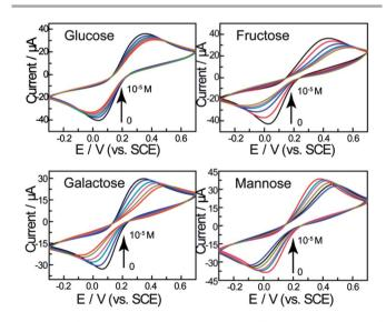
**Fig. 2** CVs of the gold electrode modified with a self-assembled monolayer of compound **1** in 0.2 M PBS (pH = 8.0) containing 5 mM Fe(CN) $_6$ <sup>3-/4-</sup> (1 : 1) with 0.1 M KNO $_3$  after treatment in the different concentrations of saccharides (from outer to inner: 0,  $10^{-6}$ ,  $3 \times 10^{-6}$ ,  $5 \times 10^{-6}$ ,  $8 \times 10^{-6}$ ,  $10^{-5}$  M) at 100 mV s<sup>-1</sup>.
