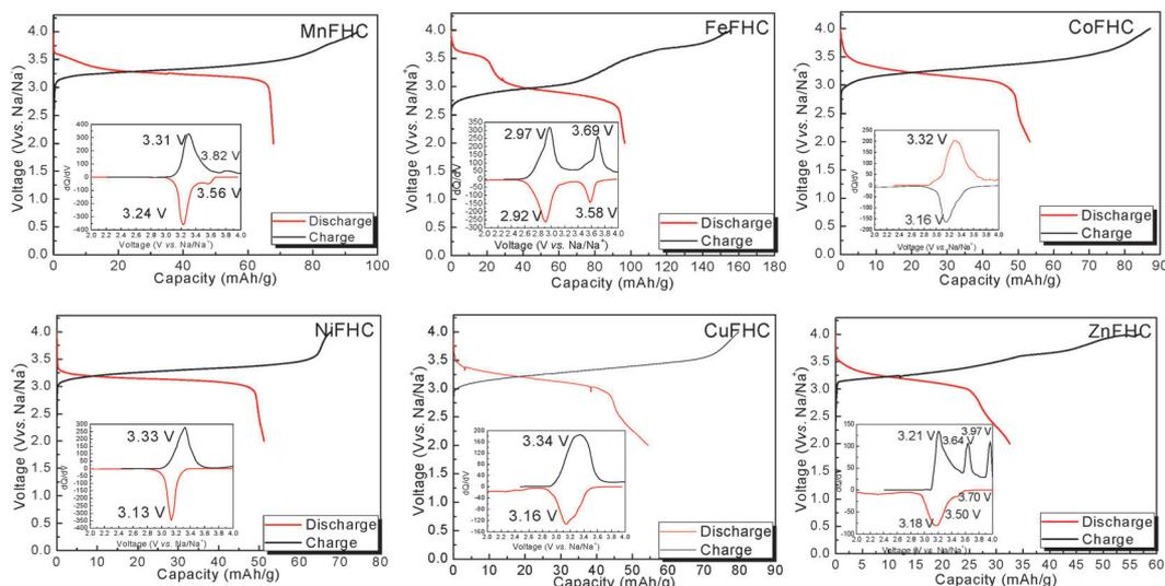
**Fig. 3** The charge-discharge curves of Prussian blue analogues  $\text{KMFe}(\text{CN})_6\text{-Na}$  cells at the third cycle with a current of  $C/20$ . Insets show their corresponding chronoamperograms.
