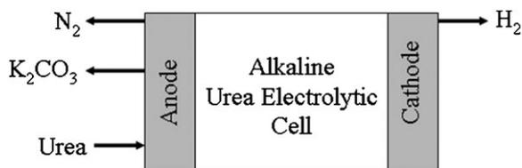
**Fig. 1** Schematic representation of the direct urea-to-hydrogen process.
