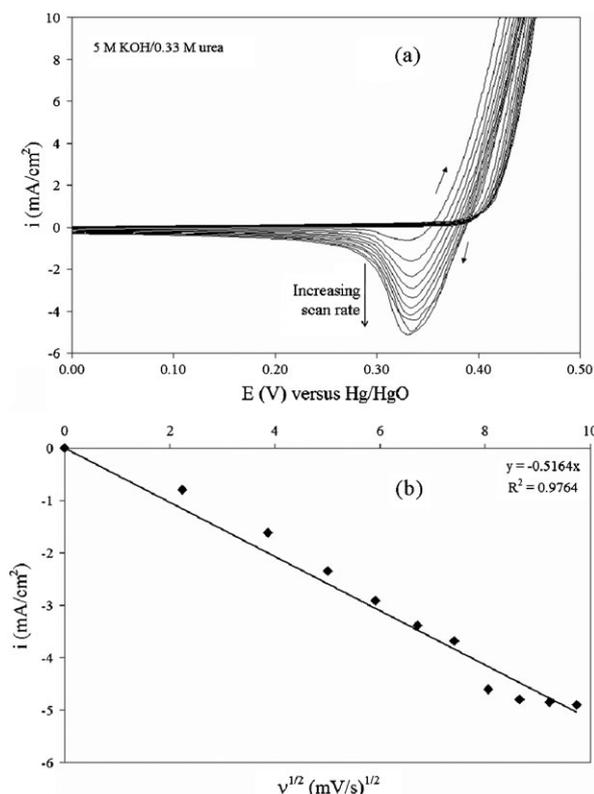
**Fig. 3** (a) Cyclic voltammograms obtained in 5 M KOH + 0.33 M urea for the NOMN electrode with various scan rates ( $\nu$ ) from 5 mV s<sup>-1</sup> to 95 mV s<sup>-1</sup>. (b) The plot of cathodic current density variation with  $\nu^{1/2}$ .
