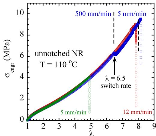
Fig. 10 Stress vs. stretch ratio curves of three NR unnotched dogbone-shaped specimens. Two of the samples were under continuous stretch at constant speed of  $5 \text{ mm min}^{-1}$  and  $12 \text{ mm min}^{-1}$ , respectively. The other was stretched at  $500 \text{ mm min}^{-1}$  till  $\lambda = 6.5$  when NR was further stretched at a slower speed of  $5 \text{ mm min}^{-1}$ .
