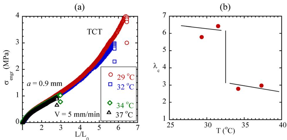
Fig. 7 (a) Stress vs. stretch ratio curves of prenotched NR with  $a = 0.9$  mm at a constant crosshead speed  $V = 5$  mm min<sup>-1</sup> at four temperatures, two below and two above the TCT. (b) NR becomes more crack resistant when  $T \leq 32$  °C, showing an abrupt TCT at ca. 32 °C.
