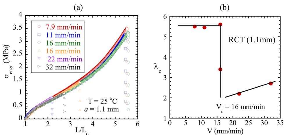
Fig. 8 (a) Stress vs. stretch ratio curves of prenotched NR with  $a = 1.1$  mm at 25 °C obtained with different crosshead speeds. (b) NR becomes more crack resistant when  $V > 16$  mm min<sup>-1</sup>, showing an abrupt RCT at ca. 16 mm min<sup>-1</sup>.
