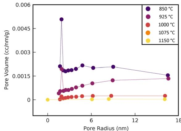
Fig. 7 Firing temperature controls pore structure in artificial clay seeds. Pore size distributions were calculated using the Barrett–Joyner–Halenda (BJH) method applied to nitrogen adsorption data from BET surface area analysis. Increasing kiln temperature reduced overall porosity and shifted the pore size distribution, enabling tunable control over imbibition dynamics in artificial seed materials.
