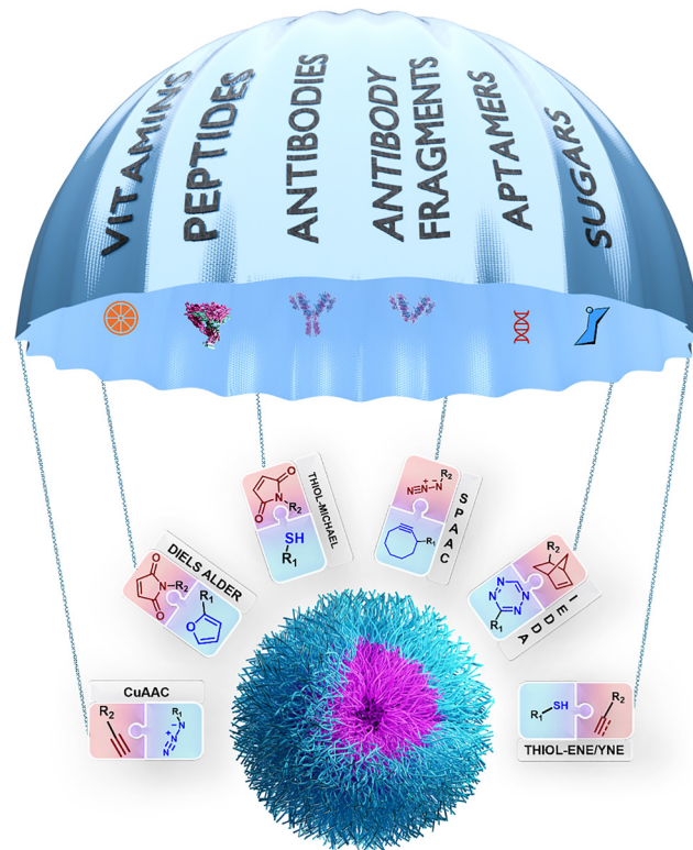
Fig. 1 Illustration of commonly employed “click” reactions to conjugate ligands onto micelles and types of ligands used for targeting. CuAAC: copper-catalyzed azide–alkyne cycloaddition, SPAAC: strain promoted azide–alkyne cycloaddition, IEDDA: inverse electron demand Diels–Alder.
