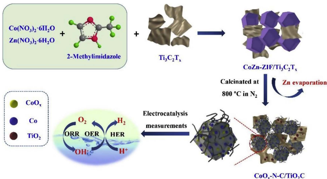
Fig. 22 Diagram illustrates the preparation process for the CoO x -N-C/TiO 2 C catalyst. 97 Reproduced from ref. 97 with permission from Elsevier Ltd, copyright © 2019.
