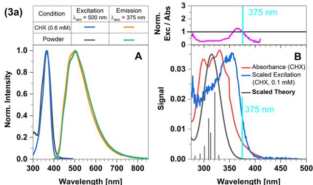
Fig. 4 Spectra of compound **3a** at 298 K (summary in Table 1). The measurements procedures are described in detail in Experimental and theoretical procedures. (A) Excitation and emission spectra in liquid cyclohexane (CHX) and powder. (B) For a qualitative comparison of the absorption properties, the excitation and the broadened DFT/MRCI spectrum were scaled to the experimental absorbance spectrum, which was corrected for baseline and scattering (eqn (3)).
