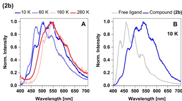
Fig. 8 (A) Steady-state luminescence spectra of **2b** in cyclohexane suspension at selected temperatures of 10 K, 60 K, 160 K, and 260 K. (B) Comparison of the steady-state spectrum of **2b** with the free ligand spectrum obtained in cyclohexane solution at 10 K. The excitation wavelength was 375 nm.
