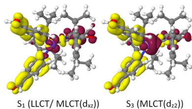
Fig. 11 Difference densities (isovalues  $\pm 0.002$ ) of the  $S_1$  (LLCT/MLCT( $d_{xz}$ )) and  $S_3$  (MLCT( $d_{zz}$ )) states of **3b** at the optimized  $S_0$  geometry. Red colour signals electron loss, yellow colour electron gain with respect to the electronic ground state density.
