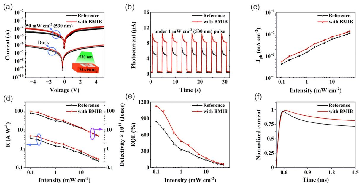
Fig. 3 (a) Dark and light  $I$ - $V$  characteristics. (b) Current-time ( $I$ - $t$ ) characteristics of the reference and BMIB-based PDs. (c) Photocurrent density ( $J_{ph}$ ), (d)  $R$  (left axis),  $D^*$  (right axis), (e) EQE and (f) normalized transient photocurrent of the reference and BMIB-based PDs under green light at 2 V.
