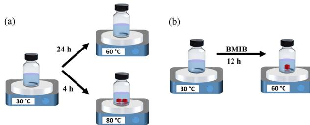
Fig. 1 Schematic of the crystallization procedure of the MAPbBr<sub>3</sub> SC (a) without and (b) with BMIB.
