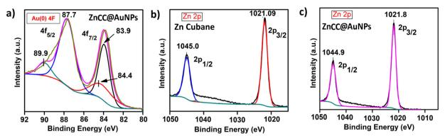
Fig. 5 XPS of (a) Au(0) 4F of ZnCC@AuNPs, (b) Zn 2p of Zn cubane, and (c) Zn 2p of ZnCC@AuNPs.
