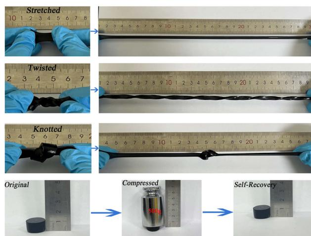
Fig. 4 Photograph of PAPP hydrogels being tested against external stimuli processes (stretched, twisted, knotted, and compressed).
