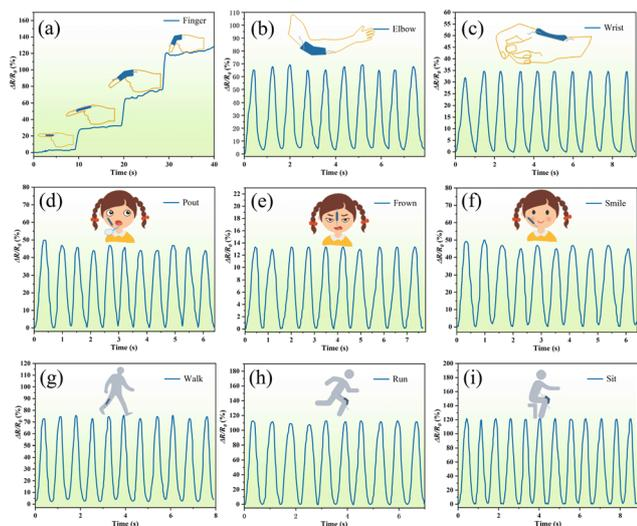
**Fig. 10** The PAPP sensors for mechanotransduction signal applications: (a) finger bending; (b) elbow bending; (c) wrist bending; (d) pouting; (e) frowning; (f) smiling; (g) walking; (h) running, and (i) sitting.
