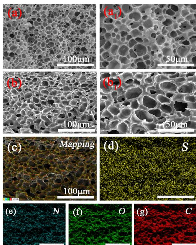
Fig. 3 The SEM images of the PAM hydrogel (a) and (a<sub>1</sub>), the PAPP hydrogel (b) and (b<sub>1</sub>), and the corresponding EDX element mapping of the PAPP hydrogel (c), including sulfur (d), nitrogen (e), oxygen (f), and carbon (g).
