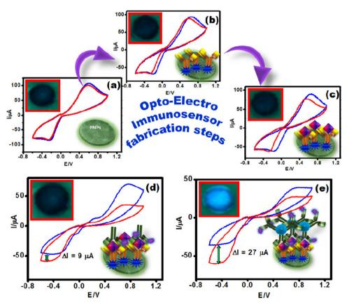
Fig. 5 Cyclic voltammetry during the construction of biosensor (a) SPE-PNPs, (b) SPE-PNPs- $^{PSA}$ Ab<sub>cap</sub>- $^{$
