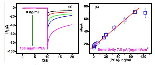
Fig. 6 (a) Amperometric curves of OCD@PSAAb2 detection probe-based PSA biosensor in the presence of 3 mM HQ and 4.5 mM H2O2 at different concentrations of PSA and (b) the calibration plot for the OCD@PSAAbupp-based PSA biosensor.
