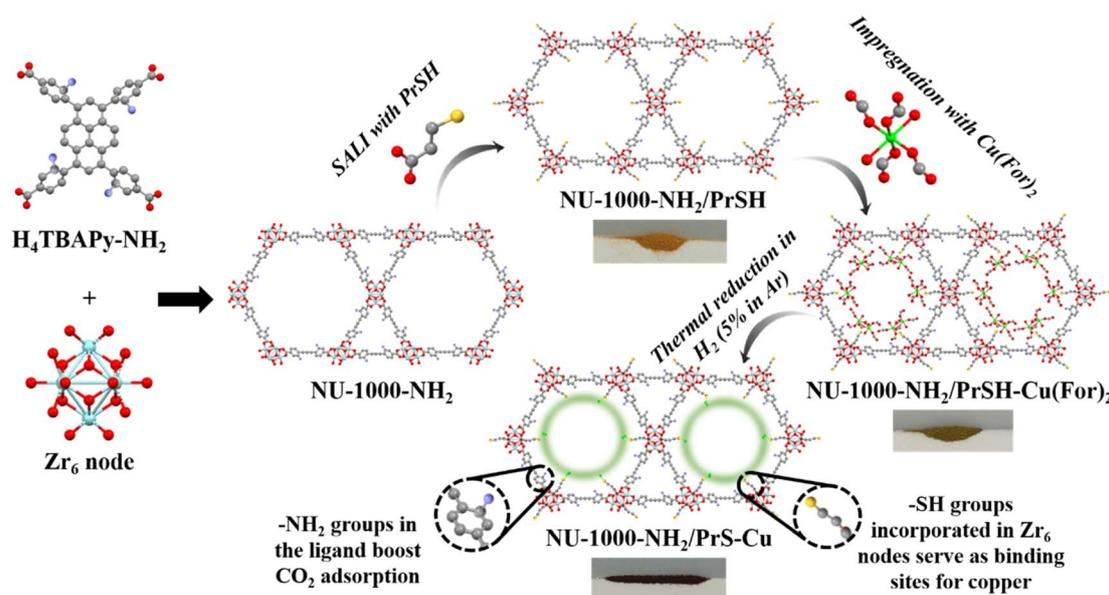
Fig. 1 Schematic representation of the followed steps to synthesize NU-1000-NH<sub>2</sub>/PrSH-Cu, emphasizing in the purpose of the installed functionalities and including the color variation of the powder.
