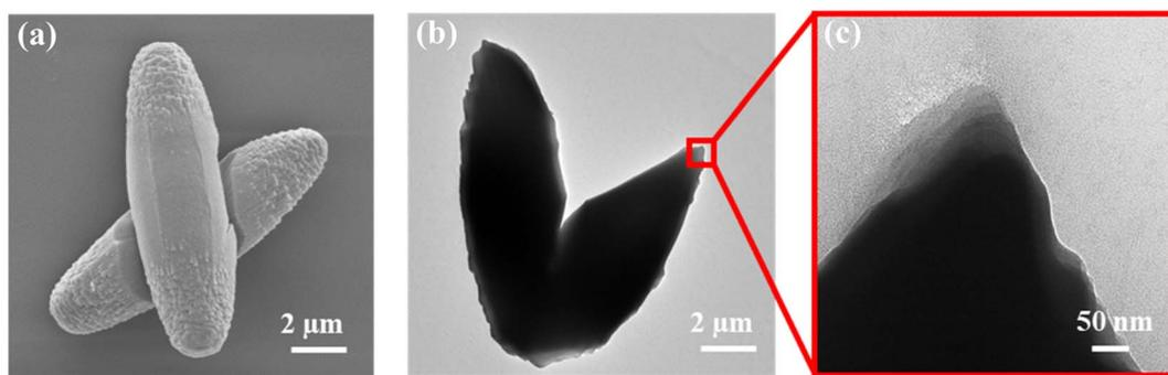
Fig. 5 Microscopic characterization of NU-1000-NH<sub>2</sub>/PrS-Cu particles: (a) SEM and (b and c) TEM micrographs.
