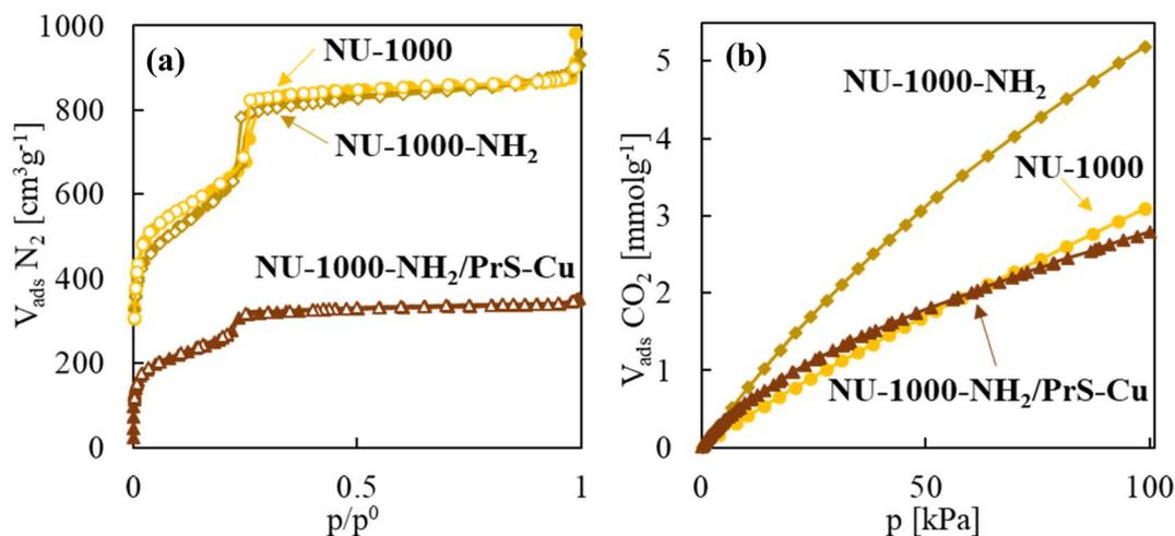
Fig. 3 Adsorption behavior: (a)  $N_2$  adsorption–desorption isotherms at  $-196\text{ }^\circ\text{C}$  and (b)  $CO_2$  adsorption isotherms at  $0\text{ }^\circ\text{C}$  of the studied samples compared to pristine NU-1000.
