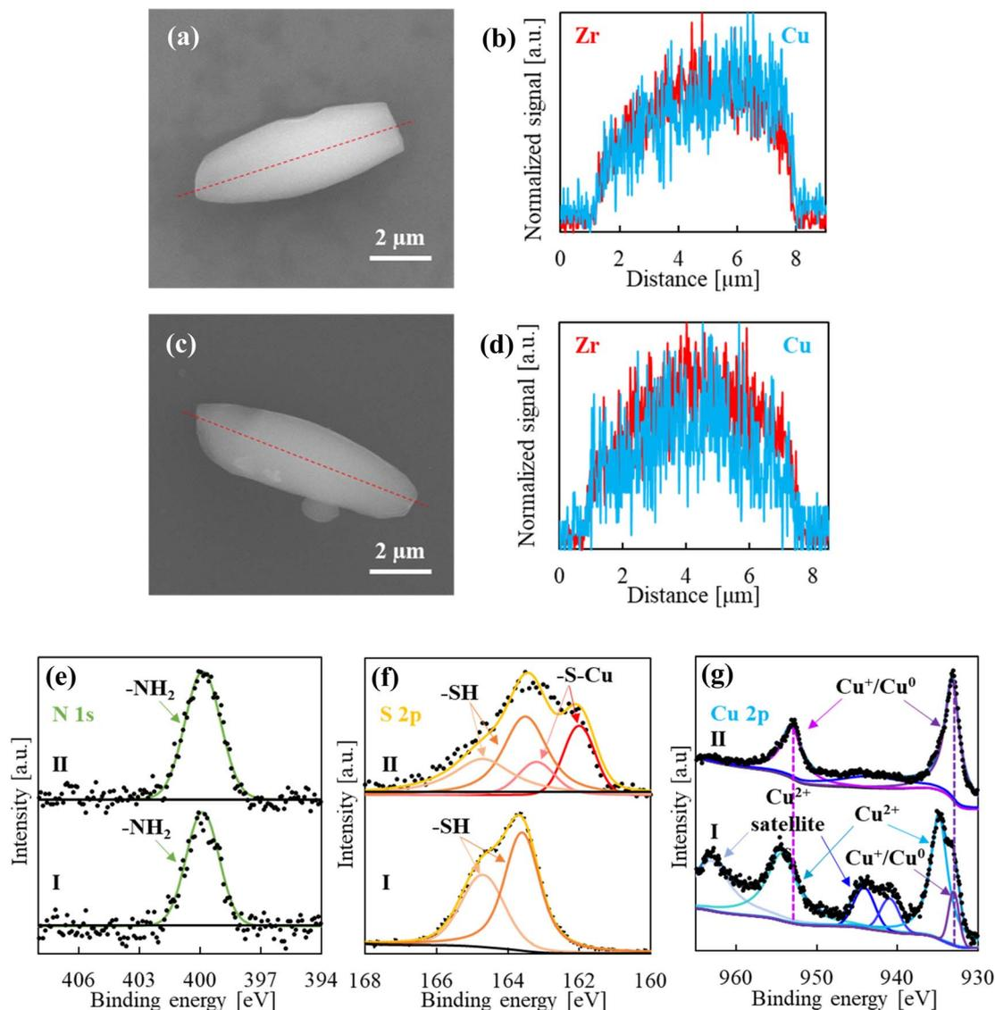
Fig. 4 Characterization before and after thermal reduction: SEM images and Zr vs. Cu EDS line scans of (a and b) NU-1000-NH<sub>2</sub>/PrSH-Cu(For)<sub>2</sub> and (c and d) NU-1000-NH<sub>2</sub>/PrS-Cu, respectively; and XPS spectra of (I) NU-1000-NH<sub>2</sub>/PrSH-Cu(For)<sub>2</sub> and (II) NU-1000-NH<sub>2</sub>/PrS-Cu in the (e) N<sub>1s</sub>, (f) S<sub>2p</sub> and (g) Cu<sub>2p</sub> regions, displaying the respective deconvoluted peaks.
