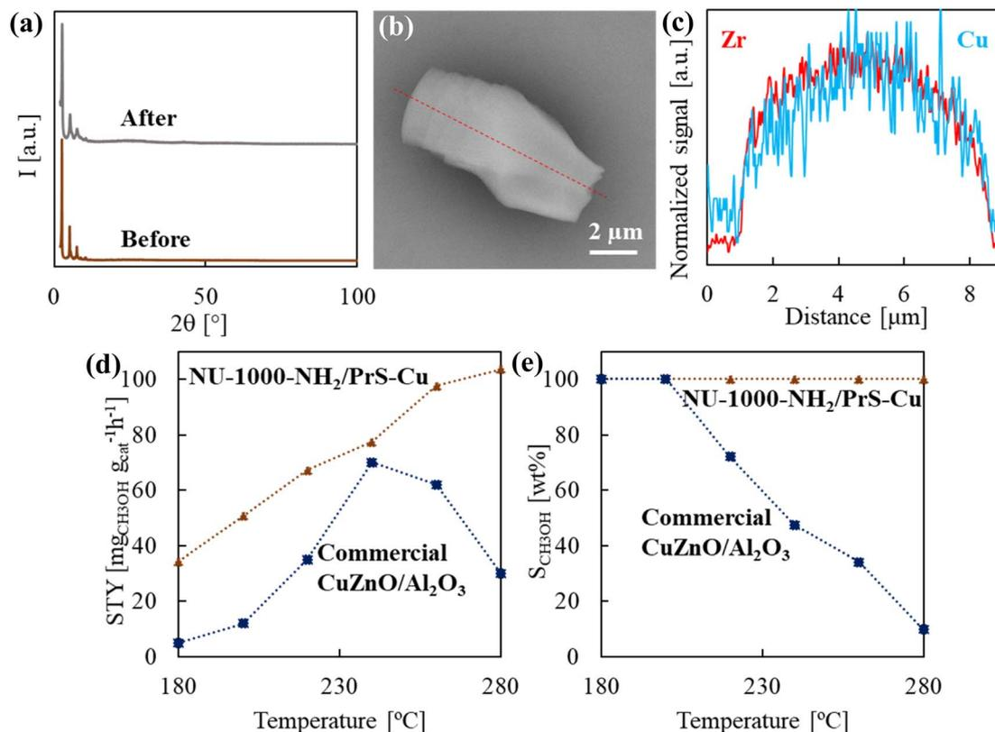
Fig. 7 Characterization and results of the sample tested for thermocatalysis: (a) PXRD of NU-1000-NH<sub>2</sub>/PrS-Cu before and after testing, (b and c) SEM image and Zr vs. Cu EDS line scan of NU-1000-NH<sub>2</sub>/PrS-Cu after testing, and (d) MeOH space-time yield (STY) and (e) MeOH selectivity ( $S_{\text{CH}_3\text{OH}}$ ) of NU-1000-NH<sub>2</sub>/PrS-Cu compared to commercial CuZnO/Al<sub>2</sub>O<sub>3</sub> at the different studied temperatures.
