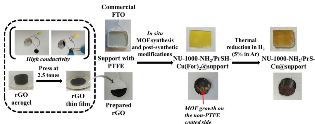
Fig. 2 Schematic representation of NU-1000-NH<sub>2</sub>/PrS-Cu@support preparation.
