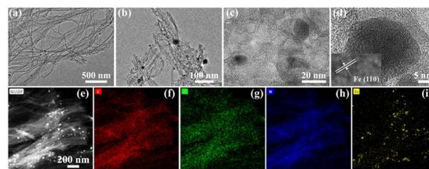
Fig. 1 (a)–(c) TEM images of sample Fe(Zn)–N–C, (d) HRTEM images showing the metallic Fe core and graphite shell, and (e)–(i) STEM image and the corresponding mapping images.
