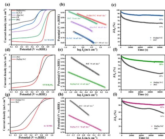
Fig. 3 (a), (d) and (g) LSV polarization, (b), (e) and (h) Tafel slope, and (c), (f) and (i) chronoamperometric plots of the as-prepared catalysts and Pt/C in 0.1 M KOH, 0.5 M H<sub>2</sub>SO<sub>4</sub>, and 0.1 M PBS solutions, respectively.
