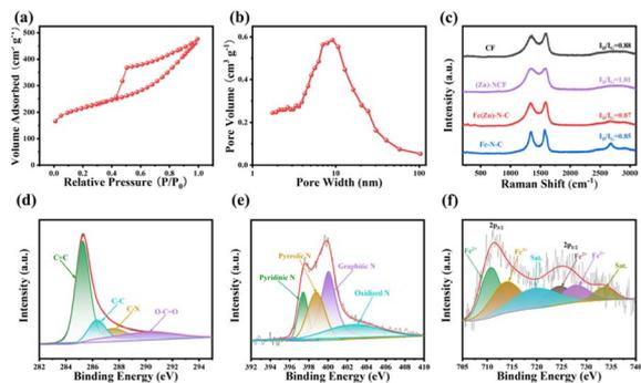
Fig. 2 (a)  $N_2$  adsorption–desorption isotherms and (b) pore diameter distribution of Fe(Zn)–N–C. (c) Raman spectra of CF, Fe–N–C, (Zn)–N–C, and Fe(Zn)–N–C. (d) High-resolution XPS spectra of C 1s, (e) N 1s, and (f) Fe 2p for the Fe(Zn)–N–C catalyst.
