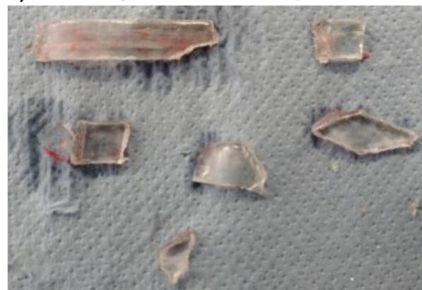
Fig. 6 Release of silver from PC by dissolution of the separation layer. (a) Shredded fragments of PC with large silver tracks on PVA layer. (b) Fragments after separation of silver by dissolution of PVA using water at ambient temperature.
