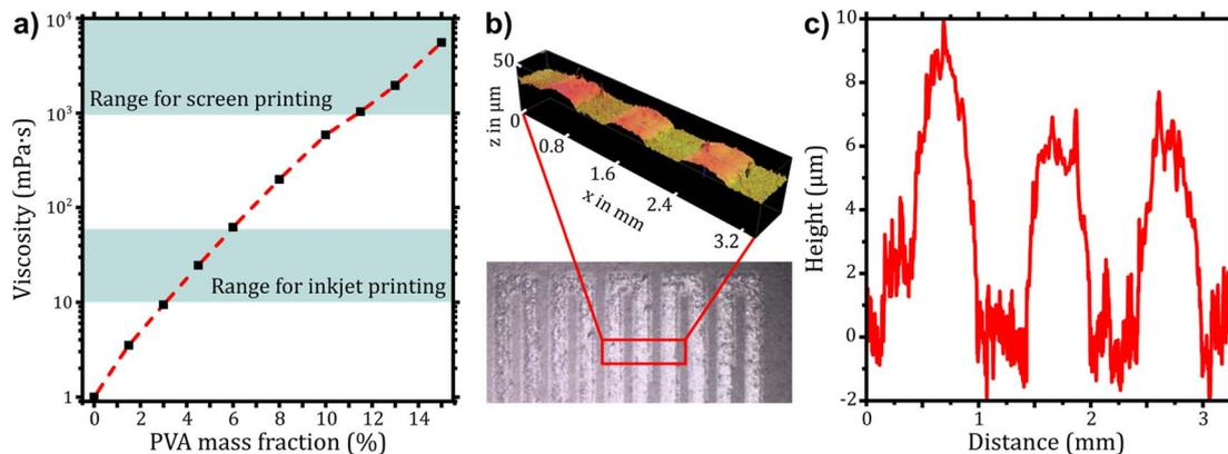
Fig. 4 Printing of PVA to prevent reduced adhesion. (a) Viscosity of aqueous solutions with different mass fractions of PVA ( $130\,000\text{ g mol}^{-1}$ ). (b) Optical microscopy image of PVA on PC and extracted 3D topography from confocal microscopy. (c) Cross section profile over three lines of the meander.
