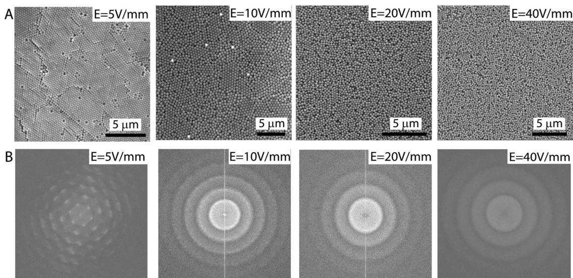
**Fig. 2** Characterization of the microstructural evolution of the colloidal assembly with the electric field change. (A) Scanning electron microscopy images of the samples electrodeposited at varying electric field strengths from  $5 \text{ V mm}^{-1}$  up to  $40 \text{ V mm}^{-1}$ . (B) Fast Fourier transformation (FFT) of the SEM images from  $5 \text{ V mm}^{-1}$  up to  $40 \text{ V mm}^{-1}$  electric field strengths. Scale bars for (A) are  $5 \mu\text{m}$ .
