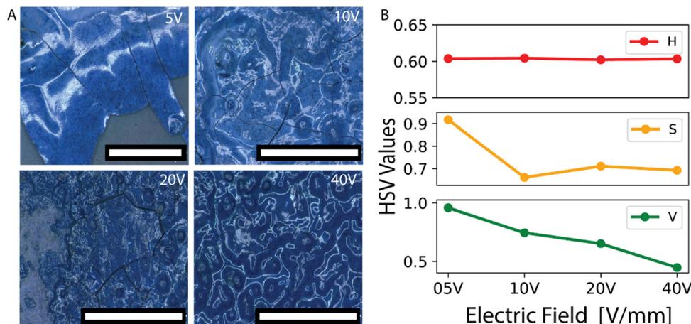
Fig. 5 Photographs and image analyses of electrodeposited films. (A) Photographs of films with 0.3% carbon black absorber at various applied electric fields from 5 to 40 V mm<sup>-1</sup>. Scale bars are 1 mm. (B) Plots of the hue (H), saturation (S), and value (V, brightness) analyses of the images from the samples in (A) demonstrate how the HSV values evolve with the change of order tuned with the electric field.
