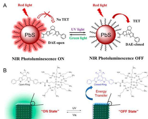
Fig. 3 (A) Photoswitchable photoluminescence of diarylethene-bound PbS QDs.<sup>54</sup> Adapted with permission from ref. 50. Copyright 2022 American Chemical Society. (B) Photoswitchable perovskite lead halide QDs coated by triethoxysilane-modified diarylethene.<sup>62</sup> Adapted with permission from ref. 57. Copyright 2020 American Chemical Society.
