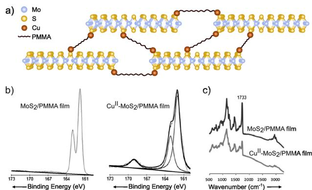
Fig. 10 (a) Scheme of the Cu<sup>II</sup>-MoS<sub>2</sub>/PMMA structure. On the bottom part, (b) S 2p core level XPS spectra of the Cu-free and Cu-coordinated MoS<sub>2</sub>/PMMA films and (c) IR of the two different species. Adapted from ref. 94, Copyright 2013, Wiley-VCH.
