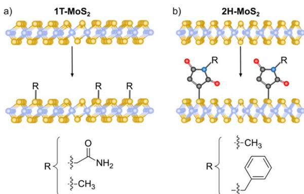
Fig. 2 Schematic representation of the MoS<sub>2</sub> functionalization strategies for (a) 1T-phase using halide derivatives and (b) 2H-phase using maleimide derivatives.
