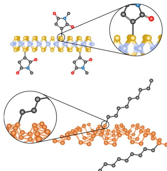
Fig. 1 Schematic representation of the covalent functionalization of 2D materials: MoS<sub>2</sub> on top and BP at the bottom.
