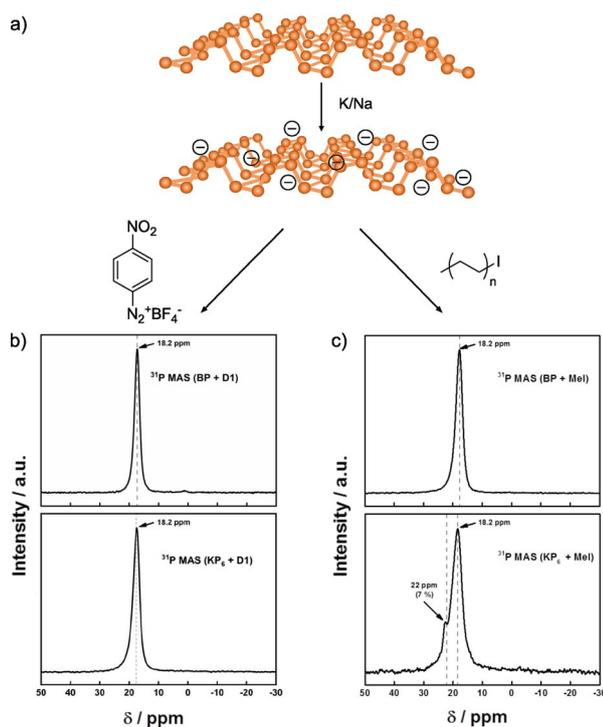
Fig. 8 (a) Scheme of the K/Na intercalation on BP. <sup>31</sup>P NMR spectra for the functionalization with (b) aryl diazonium salt and (c) alkyl iodide compounds. Both functionalizations are shown, in regard of the neutral BP or activated BP (KP<sub>6</sub> species). Adapted from ref. 142 and 128. Copyright 2020 and 2019, respectively, Wiley-VCH.
