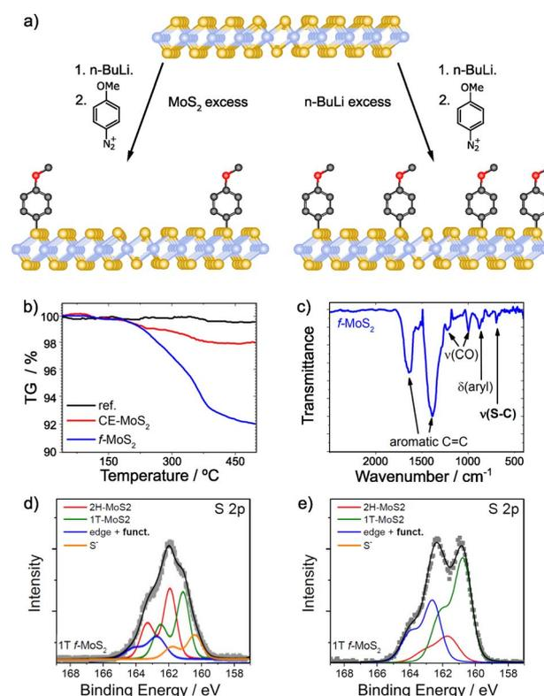
Fig. 7 (a) Scheme of the covalent functionalization of 1T-MoS<sub>2</sub>, by following two different strategies: MoS<sub>2</sub> excess (left) and *n*-BuLi excess (right); TGA and IR spectra for functionalized MoS<sub>2</sub> in the presence of MoS<sub>2</sub> excess are shown on (b) and (c) respectively; S 2p core level XPS spectra of the different materials: (d) MoS<sub>2</sub> excess and (e) *n*-BuLi excess. Adapted with permission from ref. 135. Copyright 2015 American Chemical Society.
