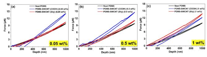
Fig. 3 Loading—unloading plots from nanoindentation analysis of the test structures at different SWCNT loadings on PDMS: (a) 0.05 wt%, (b) 0.5 wt% and (c) 1 wt%. The curves indicate the resistance shown by the samples to indentation force and the area under the curves indicate the plastic deformation undergone by the samples.
