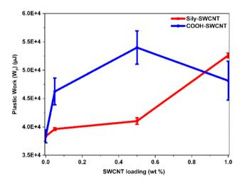
Fig. 4 Plastic work  $(W_{\rm p})$  undergone by PDMS-SWCNT composite samples during nanoindentation analysis.
