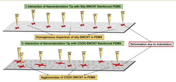
Fig. 8 Schematic of the interaction of nanoindentation tip with (I) sily-SWCNT reinforced PDMS, and (II) COOH-SWCNT reinforced PDMS.
