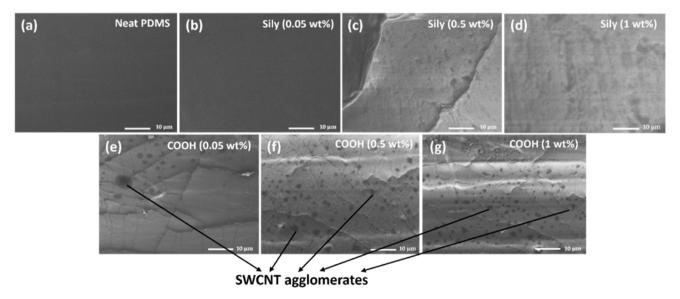
Fig. 2 Cross-sectional FESEM analysis of the test structures: (a) neat PDMS, (b) PDMS-SWCNT (sily, 0.05 wt%), (c) PDMS-SWCNT (sily, 0.5 wt%), (d) PDMS-SWCNT (sily, 1 wt%) (e) PDMS-SWCNT (COOH, 0.05 wt%), (f) PDMS-SWCNT (COOH, 0.5 wt%), (g) PDMS-SWCNT (COOH, 1 wt%).
