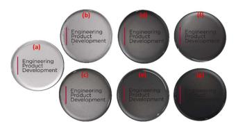
Fig. 1 Photographic images of the fabricated test structures: (a) neat PDMS, (b) PDMS–SWCNT (sily, 0.05 wt%), (c) PDMS–SWCNT (COOH, 0.05 wt%), (d) PDMS–SWCNT (sily, 0.5 wt%), (e) PDMS–SWCNT (COOH, 0.5 wt%), (f) PDMS–SWCNT (sily, 1 wt%), (g) PDMS–SWCNT (COOH, 1 wt%).
