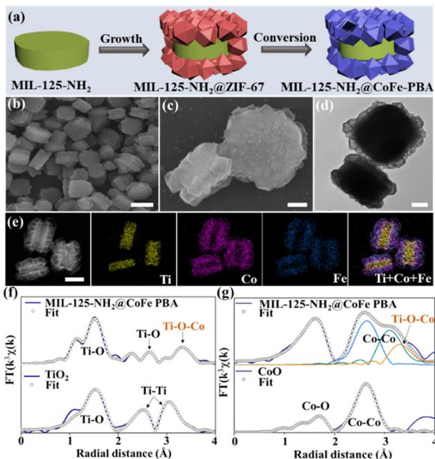
**Fig. 10** (a) Illustration of the synthesis process of MIL-125-NH<sub>2</sub>@CoFe PBA. (b and c) SEM, (d) TEM, (e) HAADF-STEM and the corresponding elemental mapping images. Scale bars are: (b), 1 μm; (e), 500 nm; and (c and d), 200 nm. (f) Ti coordination environments of MIL-125-NH<sub>2</sub>@CoFe PBA and TiO<sub>2</sub> and (g) Co coordination environments of MIL-125-NH<sub>2</sub>@CoFe PBA and CoO. Reprinted with permission from ref. 44. Copyright 2023 Wiley-VCH.
