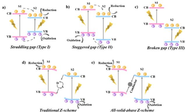
**Fig. 1** Band structures and charge transfer directions in (a) straddling gap (type I), (b) staggered gap (type II), (c) broken gap (type III), (d) traditional Z-scheme, and (e) all-solid-state Z-scheme heterojunctions.
