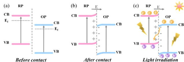
**Fig. 2** Graphical illustration of the charge migration process of S-scheme heterojunctions. (a) before contact; (b) after contact; and (c) photogenerated charge carrier transfer under light irradiation.
