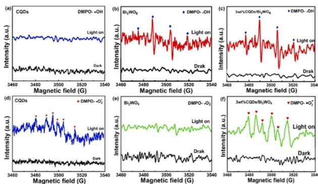
Fig. 6 EPR signals of CQDs,  $\text{Bi}_2\text{WO}_6$ , and 3 wt% CQDs/ $\text{Bi}_2\text{WO}_6$  for DMPO-OH (a, b and c) and DMPO- $\text{O}_2^-$  (d, e, and f). Reprinted with permission from ref. 79. Copyright 2023 Elsevier.
