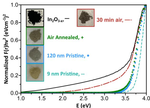
Fig. 4 Kubelka–Munk plot of the black  $\text{In}_2\text{O}_{3-x}$ , 30 minutes of air flow, air annealed, 120 nm, and 9 nm nanoparticles using  $r = \frac{1}{2}$  for the direct transition. Inset shows dried powders of each of the measured nanoparticles.
