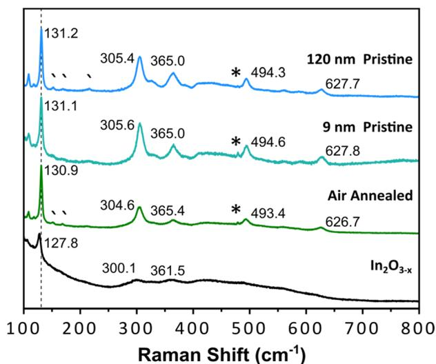
**Fig. 5** Raman spectra of the black  $\text{In}_2\text{O}_{3-x}$  air annealed, 120 nm, and 9 nm nanoparticles. The observed Raman modes are labeled with their respective wavenumbers with smaller modes in the 120 nm and air annealed nanoparticles denoted by ' '. The vertical line crosses the peak at  $\sim 130\text{ cm}^{-1}$  and shows a red-shift in the spectrum for the black  $\text{In}_2\text{O}_{3-x}$  sample. The asterisks denote signal from the room lighting.
