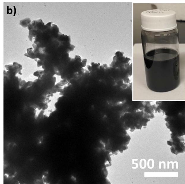
**Fig. 1** (a) PXRD of the obtained black  $\text{In}_2\text{O}_{3-x}$  compared to the simulated pattern for bixbyite  $\text{In}_2\text{O}_3$ . (b) TEM image of the black  $\text{In}_2\text{O}_{3-x}$  showing dense agglomerations. The inset shows a picture of the particles dispersed in toluene.
