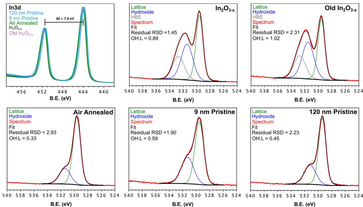
**Fig. 6** XPS spectra of the black  $\text{In}_2\text{O}_{3-x}$ , aged black  $\text{In}_2\text{O}_{3-x}$ , air annealed, 9 nm pristine, 120 nm pristine, and commercial samples. Each spectrum was fit with lattice and surface hydroxyl groups, while the black  $\text{In}_2\text{O}_{3-x}$  samples displayed an additional HBE feature. The Survey scans of each material are found in Fig. S24<sup>†</sup> and peak fitting parameters for the O 1s fitting are found in Table S3.<sup>†</sup>
