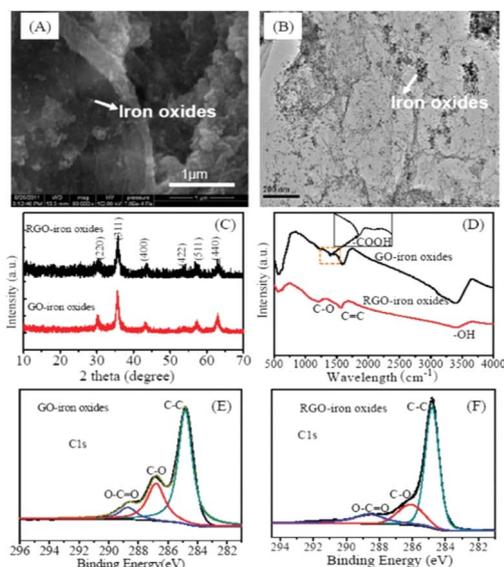
Fig. 10 SEM (A) and TEM (B) images, XRD patterns (C), FTIR spectra (D), and high-resolution C 1s (E and F) XPS of GO-Fe<sub>3</sub>O<sub>4</sub> NC and rGO-Fe<sub>3</sub>O<sub>4</sub> NC hybrid materials. This figure has been reproduced from ref. 244 with permission from the Royal Society of Chemistry, Copyright 2012.
