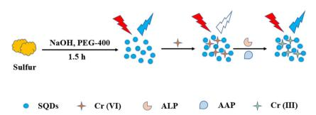
Fig. 4 Schematic diagram of the synthesis of SQDs and determination of ALP. From ref. 83 with permission. Copyright 2022, MDPI.
