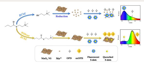
Fig. 8 Schematic illustration of the assay for the detection of BChE. From ref. 106 with permission. Copyright 2021, Springer.
