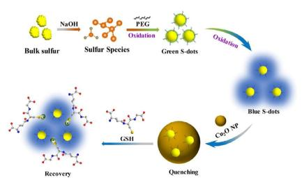
Fig. 3 Schematic illustration of the fluorescence assay for GSH. From ref. 76 with permission. Copyright 2022, Elsevier.
