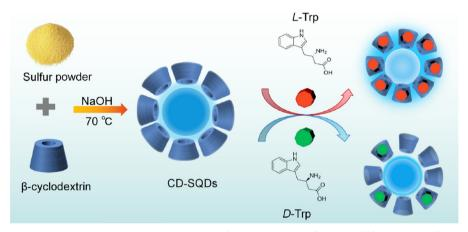
Fig. 12 Schematic illustration of the sensing of L and p-Trp. From ref. 132 with permission. Copyright 2023, American Chemical Society.
