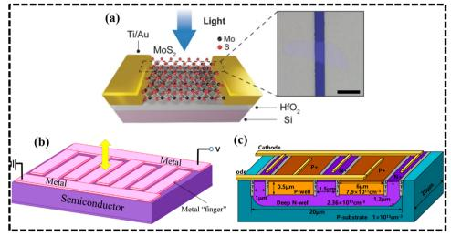
Fig. 12 (a) High responsivity in MoS<sub>2</sub> phototransistors based on charge trapping HfO<sub>2</sub> dielectrics. 155 (b) avalanche photo diode. 156 and (c) MoS<sub>2</sub> phototransistors. Reprinted with permission from ref. 157
