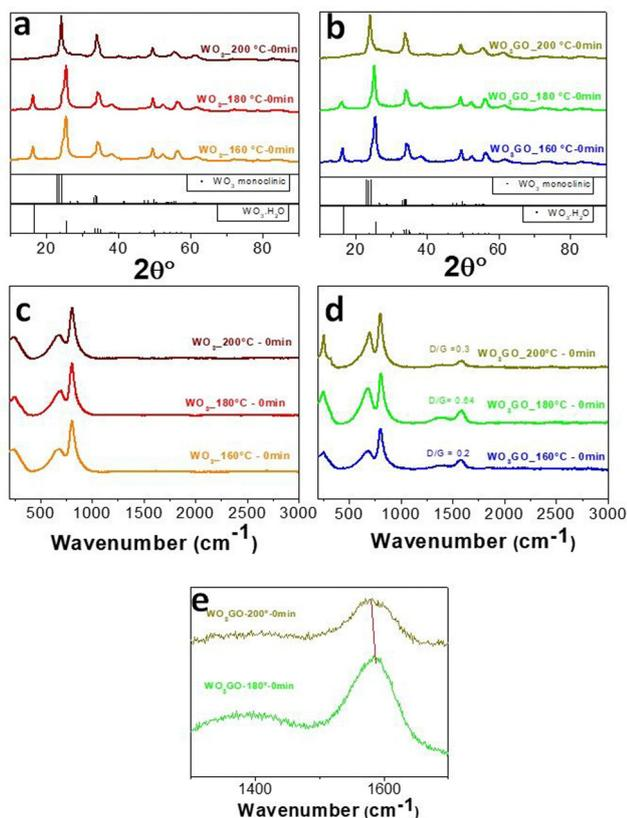
Fig. 2 XRD of pristine  $\text{WO}_3$  samples (a) and  $\text{WO}_3$  modified with GO (b). Raman spectra of pristine (c) and GO-modified samples (d). Enlarged view of the graph (d), emphasizing the shift of the G band between  $\text{WO}_3\text{GO}-180$  °C-0 min and  $\text{WO}_3\text{GO}-200$  °C-0 min (e).
