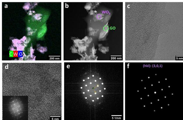
**Fig. 5** (a) HAADF-STEM micrograph of  $\text{WO}_3\text{GO}_{200\text{ }^\circ\text{C-10 min}}$  with the elemental map obtained from  $W_{L\alpha}$ ,  $O_{K\alpha}$ , and  $C_{K\alpha}$ . (b) HAADF image with selected regions of  $\text{WO}_3$  and GO and (c) HRTEM images of GO and (d)  $\text{WO}_3$  with a fast-Fourier-transform pattern (FFT – inset). (e) FFT pattern fitted with the schematic diagram of monoclinic  $\text{WO}_3$  (301) and (f) calculated diffraction pattern (301).
