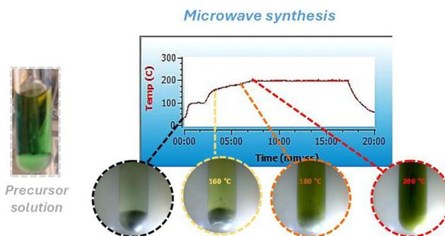
Fig. 1 Temperature vs. reaction time graph of the microwave synthesis of WO<sub>3</sub>, along with images of the reaction solutions.
