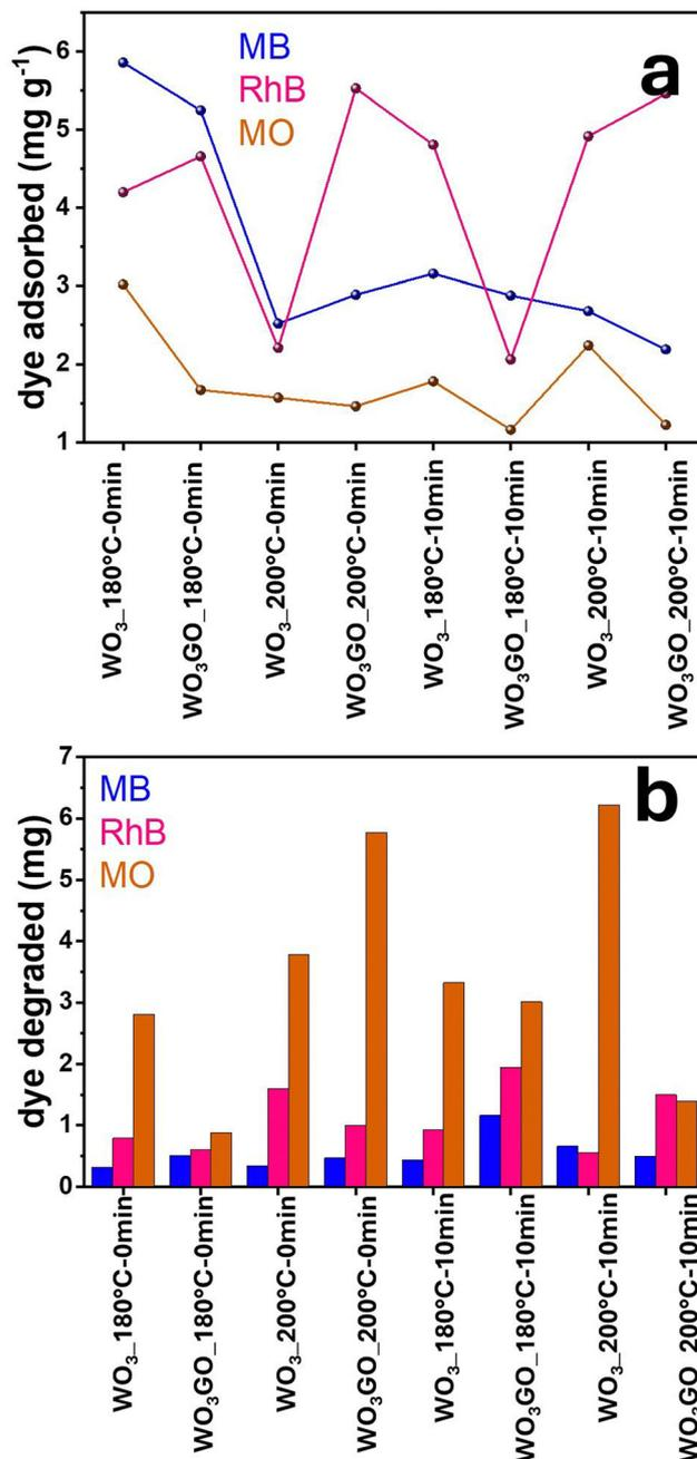
**Fig. 8** Correlation between the MB, RhB and MO mass adsorbed onto each catalyst after 1440 min of adsorption in the dark (a) and the mass of dye degraded after 60 min of simulated sunlight irradiation (b).
