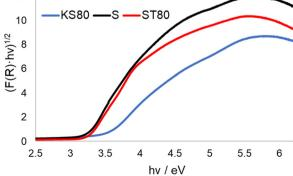
Fig. 3 Diffuse reflectance UV-Vis analysis of titanosilicate samples KS80, S and ST80. (A) Kubelka-Munk plots, (B) Tauc plots
