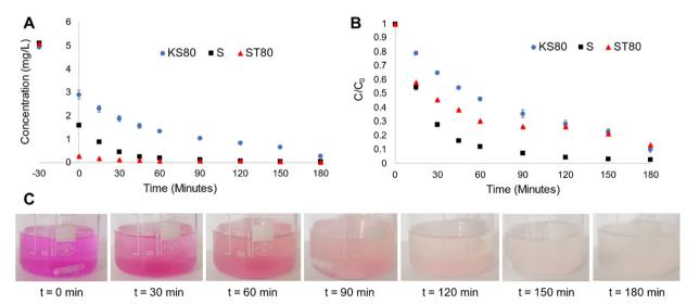
Fig. 6 Rh B degradation study using titanosilicates KS80, S and ST80. (A) Rh B concentration vs. time plots, (B) normalized results  $C/C_0$  vs. time (i.e., final/initial Rh B concentration). (C) Images of Rh B degradation taken throughout the reaction, using sample ST80 as catalyst.
