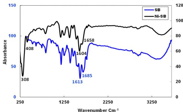
Fig. 2 FTIR spectrum for SB and Ni(II)-SB.
