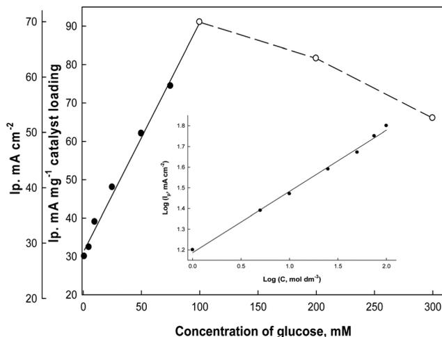
Fig. 10 Effect of glucose concentrations on the oxidation peak current densities of glucose in 0.5 M NaOH at 0.02 V s<sup>-1</sup> (from cyclic voltammograms, not presented), and the inset plot represents the logarithmic relationship between the concentrations and the oxidation peak current densities.
