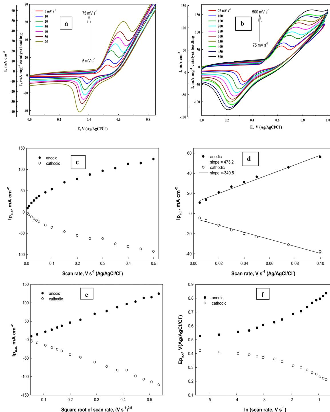
Fig. 9 (a) and (b) Cyclic voltammograms of the Ni(II)-SB/C electrode at different scan rates in 0.5 M NaOH. (c) and (d) The dependence of anodic (the solid dots) and cathodic (the open dots) peak currents on the scan rates. (e)  $I_{pa,c}$  vs. square root of scan rates and (f) dependence of peak potentials on the natural logarithm of the scan rates.
