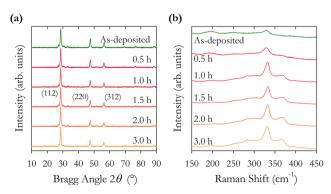
Fig. 7 (a) XRD spectra for thin films annealed at 500  $^{\circ}$ C as a function of annealing time. (b) Raman spectra for as-synthesised CZTS particles and films annealed at 500  $^{\circ}$ C for different durations using an excitation wavelength of 785 nm.
