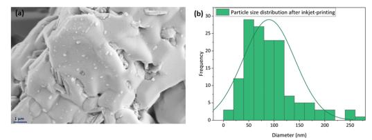
Fig. 11 (a) Surface SEM image with a high magnification of 8.66k× from the 100-layer inkjet-printed sample and (b) CuFe<sub>2</sub>O<sub>4</sub> nanoparticle size distribution on its surface, analyzed using ImageJ software.
