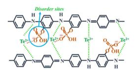
Fig. 5 Charge transport mechanism in Te-PANI. [Reproduced from ref. 34, with permission from Springer Nature, Copyright 2023.]
