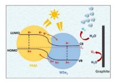
Fig. 15 Energy band structure with HER and OER in  $PANI/WSe_2$  nanohybrid. [Reproduced from ref. 76, with permission from Elsevier, Copyright 2021.]
