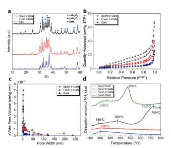
Fig. 2 (a) XRD patterns of the GaN, fresh and spent Ir/GaN catalysts. (b)  $N_2$  adsorption isotherm profiles of the GaN, fresh and spent Ir/GaN catalysts. (c) Pore size distributions of the GaN, fresh and spent Ir/GaN samples. (d)  $NH_3$ -TPD profiles of all fresh and spent samples.
