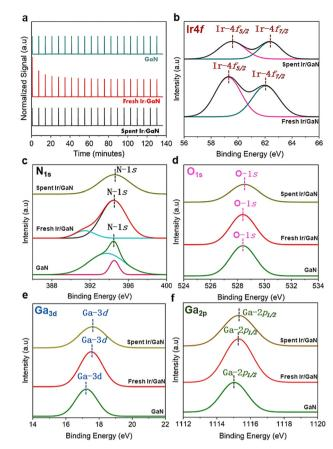
Fig. 3 (a) CO pulse chemisorption profiles of the GaN, fresh and spent Ir/GaN catalysts. (b) High-resolution XPS spectra of the Ir4f and fresh and spent Ir/GaN catalysts. (c) XPS spectral surveys of  $N_{1s}$ . (d) XPS spectral surveys of  $O_{1s}$ . (e) XPS spectral surveys of Ga<sub>3d</sub>. (f) XPS spectral surveys of Ga<sub>2D</sub>.
