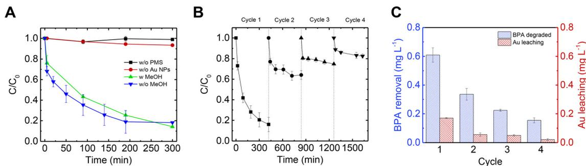
**Fig. 5** Peroxymonosulfate (PMS) activation for bisphenol A (BPA) degradation. (A) Removal of BPA with PMS and Au nanoparticles in dispersion.  $[BPA]_0 = 1 \text{ mg L}^{-1}$ ;  $[PMS]_0 = 0.2 \text{ mM}$ ;  $[Au \text{ NPs}]_0 = 0.015 \text{ g L}^{-1}$ . (B) Removal of BPA with Au nanoparticle-embedded mucin nanofibers (in the presence of PMS) over four cycles. (C) BPA removal by Au-embedded nanofibers (blue) and Au leaching (red) for each cycle in (B).
