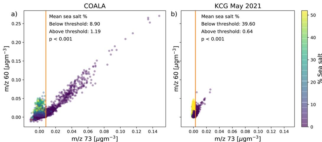
Fig. 6 Concentrations of  $m/z$  60 and  $m/z$  73 shaded by the percentage of total OA concentration from each location's sea salt factor at COALA (a) and KCG in May 2021 (b).  $p$ -Values quoted are the result of independent  $t$ -tests comparing mean percentages of sea salt concentration above and below  $m/z$  73 threshold concentration at each site.
