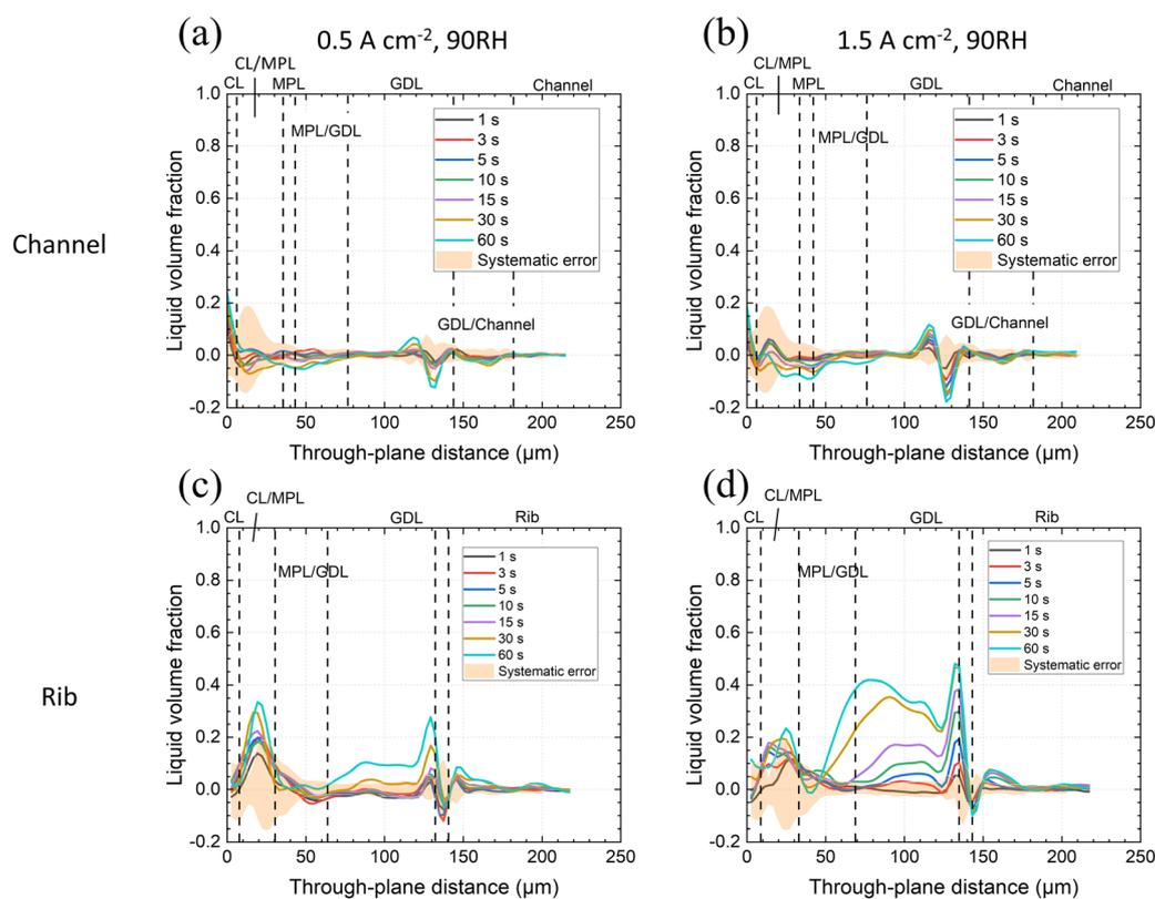
Fig. 6 Average liquid volume fraction (LVF) of product water in CL, MPL and GDL of the *operando* Li100-cell with 90% RH feed gases; LVF profiles at are given at indicated times after the start of constant current operation are given with estimated non-random error plotted as orange shade at (a) and (b) 0.5  $\text{A cm}^{-2}$  & 1.5  $\text{A cm}^{-2}$  under the channel, (c) and (d) 0.5  $\text{A cm}^{-2}$  & 1.5  $\text{A cm}^{-2}$  under the rib.
