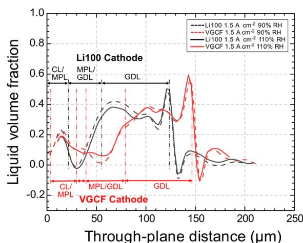
Fig. 9 LVF comparison of the Li100- and VGCF-cells at 1.5 A cm<sup>-2</sup> current density under the rib at 60 s for the RH = 90% and 110% conditions. The LVF profiles are aligned at the CL/MPL interface, and the respective domains (CL/MPL, MPL/GDL and GDL) for cells with both are specified with dashed red or black lines. Note that the thickness of the GDLs of the two cells is different, by ca. 17 μm (when uncompressed).
