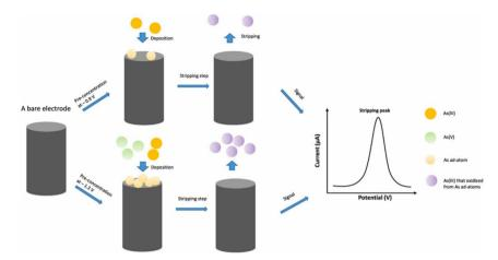
Fig. 16 The total arsenic concentration measured by deposition at -1.3 V while the As(III) measured at -0.9 V on gold macroelectrodes based on the underpotential deposition (UPD) of As ad-atoms<sup>131</sup> (reprinted from ref. 131; Copyright (2022), with permission from Elsevier).
