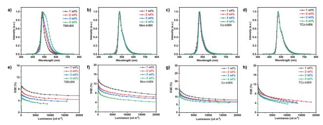
Fig. 4 (a-d) The EL spectra and (e-h) the EQE-luminance curves of the OLED devices based on TMInBN, Mes-InBN, Cz-InBN, and TCz-InBN.
