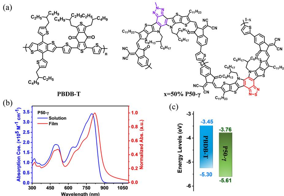
Fig. 1 (a) Molecular structures of PBDB-T and P50- $\gamma$ . (b) Absorption spectra of P50- $\gamma$  in dilute chloroform ( $<10^{-6}$  mol L $^{-1}$ ) and thin film. (c) Energy levels of PBDB-T and P50- $\gamma$ .
