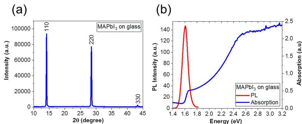
Fig. 1 (a) XRD pattern and (b) PL (red line) and absorption (blue line) spectra of a MAPbI<sub>3</sub> film on glass substrate.
