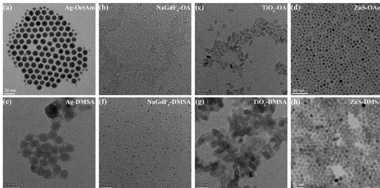
Fig. 2 TEM images of (a) Ag-OctAm, (b) NaGdF<sub>4</sub>-OA, (c) TiO<sub>2</sub>-OA, (d) ZnS-OAm, (e) Ag-DMSA, (f) NaGdF<sub>4</sub>-DMSA, (g) TiO<sub>2</sub>-DMSA and (h) ZnS-DMSA.
