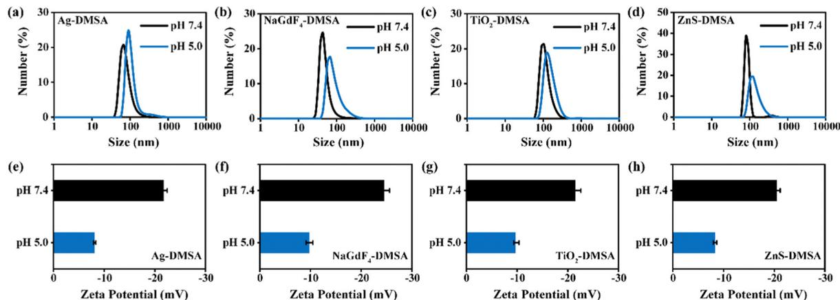
Fig. 5 (a)–(d) Hydrodynamic radius values of (a) Ag-DMSA, (b) NaGdF<sub>4</sub>-DMSA, (c) TiO<sub>2</sub>-DMSA and (d) ZnS-DMSA each under two different pH conditions. (e)–(h) Zeta potentials of (e) Ag-DMSA, (f) NaGdF<sub>4</sub>-DMSA, (g) TiO<sub>2</sub>-DMSA and (h) ZnS-DMSA each under two different pH conditions.
