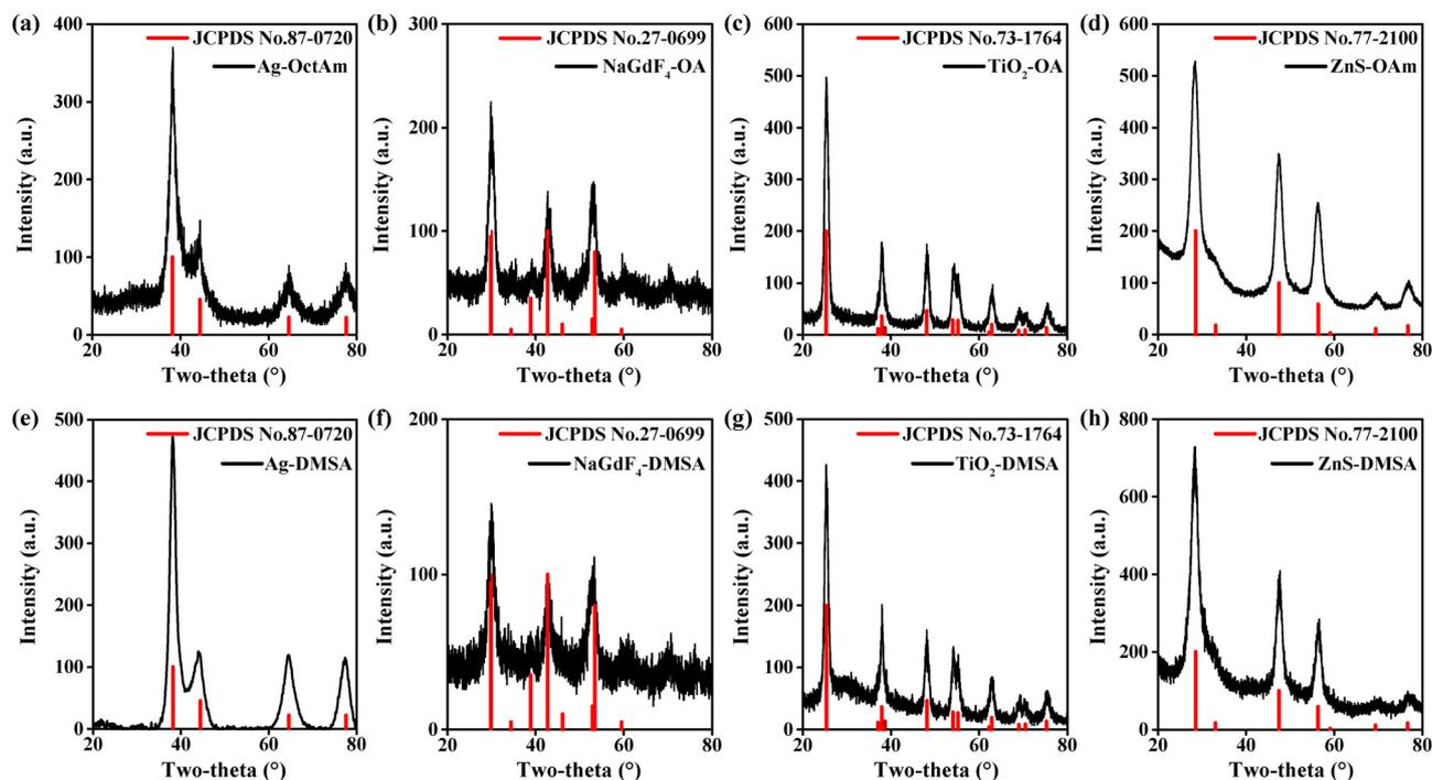
Fig. 3 XRD patterns of (a) Ag-OctAm, (b) NaGdF<sub>4</sub>-OA, (c) TiO<sub>2</sub>-OA, (d) ZnS-OAm, (e) Ag-DMSA, (f) NaGdF<sub>4</sub>-DMSA, (g) TiO<sub>2</sub>-DMSA and (h) ZnS-DMSA.
