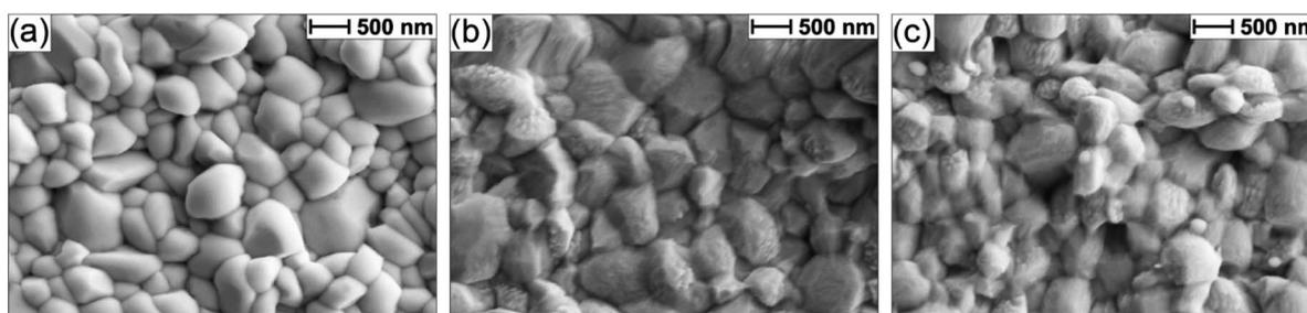
Fig. 2 SEM images for an FTO/Ti/Au/ $\text{Sb}_2\text{Se}_3$  sample (a) untreated, (b) etched *via* (NH<sub>4</sub>)<sub>2</sub>S, and (c) etched *via* (NH<sub>4</sub>)<sub>2</sub>S + CuCl<sub>2</sub> treatment.
