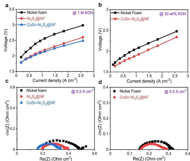
Fig. 6 Electrochemical results of alkaline water electrolysis cells (with NF, Ni<sub>3</sub>S<sub>2</sub>@NF, and CoSn-Ni<sub>3</sub>S<sub>2</sub>@NF electrodes). Current–voltage curves of alkaline cells under (a) 1 M KOH at 55 °C and (b) 30 wt% KOH solution at 80 °C. EIS curves of alkaline cells at 0.5 A cm<sup>-2</sup> under (c) 1 M KOH at 55 °C and (d) 30 wt% KOH solution at 80 °C.
