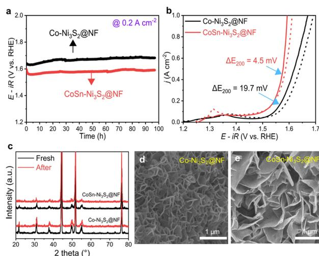
Fig. 5 Long-term stability of OER catalysts. (a) Durability tests of Co-Ni<sub>3</sub>S<sub>2</sub>@NF and CoSn-Ni<sub>3</sub>S<sub>2</sub>@NF catalysts under 0.2 A cm<sup>-2</sup> for 97 h. (b) Changes of OER activity curves of catalysts after 1000th cycling test between 1.25 V and 1.65 V. (c) XRD patterns of catalysts before and after durability test. FE-SEM image of (d) Co-Ni<sub>3</sub>S<sub>2</sub>@NF and (e) CoSn-Ni<sub>3</sub>S<sub>2</sub>@NF catalysts after durability test.
