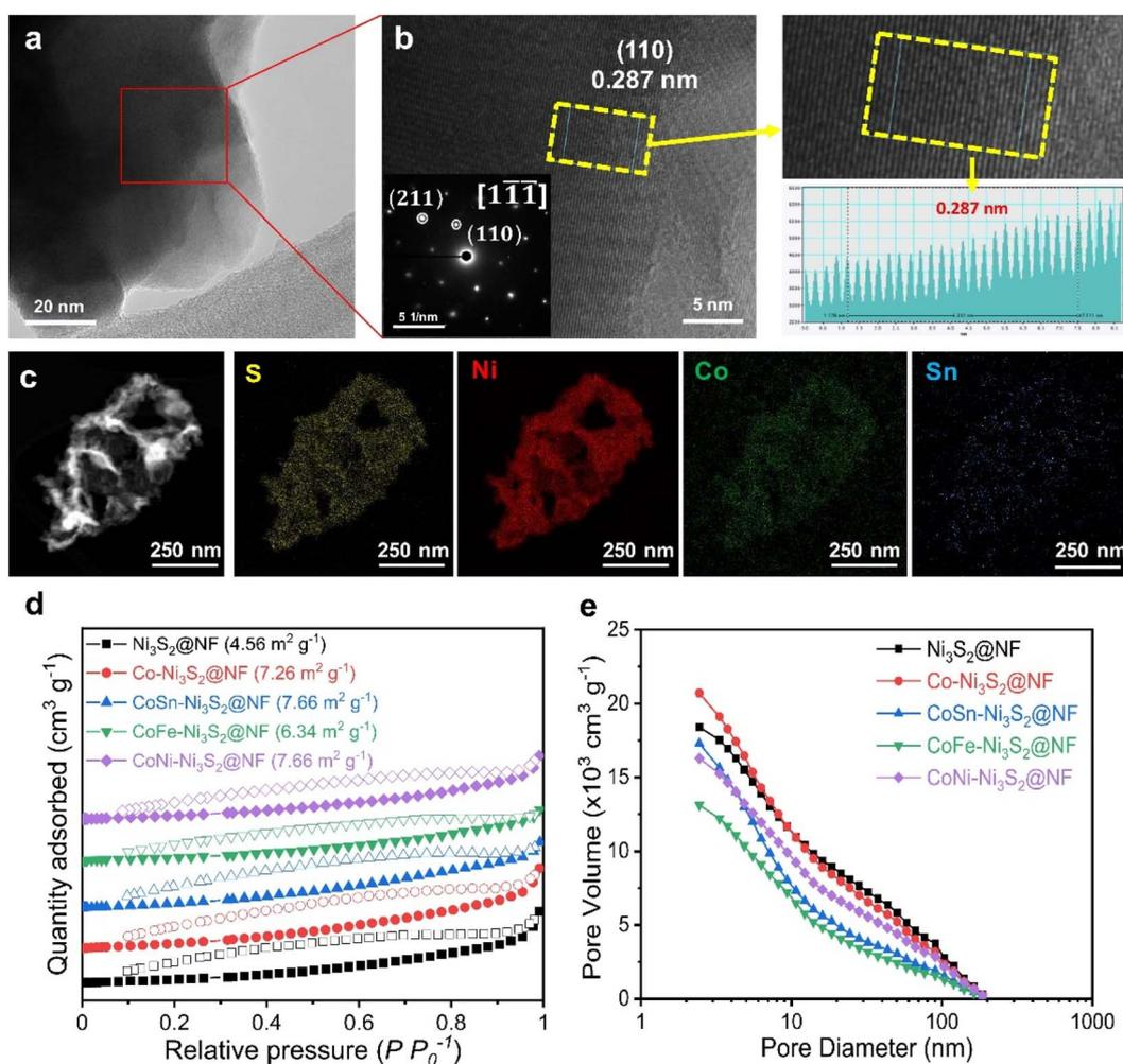
Fig. 3 Physicochemical analysis of catalysts. (a) HRTEM image and (b) enlarged image with SAED pattern of CoSn-Ni<sub>3</sub>S<sub>2</sub>@NF. The right inset shows an atomic resolution image of yellow dashed box. (c) EDX spectra of each element of CoSn-Ni<sub>3</sub>S<sub>2</sub>@NF. (d) Nitrogen adsorption-desorption isotherms and (e) total pore volume and pore size of Ni<sub>3</sub>S<sub>2</sub>@NF, Co-Ni<sub>3</sub>S<sub>2</sub>@NF, and CoSn-Ni<sub>3</sub>S<sub>2</sub>@NF.
