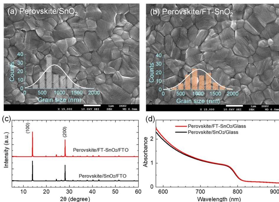
**Fig. 3** Top-view SEM image of the perovskite layer coated on (a) bare SnO<sub>2</sub> and (b) FT-SnO<sub>2</sub>. Insets show grain size distribution. (c) XRD patterns of the perovskite films formed on SnO<sub>2</sub>- and FT-SnO<sub>2</sub>-coated FTO substrate. (d) Absorbance of the perovskite films deposited on SnO<sub>2</sub>- and FT-SnO<sub>2</sub>-coated glass substrate.
