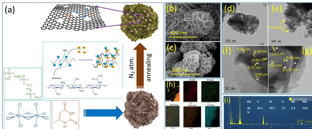
**Fig. 1** (a) Preparation of  $\text{NbMo}_6\text{S}_8/\text{NC}$  via the hydrothermal process. Morphological characterization of  $\text{NbMo}_6\text{S}_8$  and  $\text{NbMo}_6\text{S}_8/\text{NC}$ : SEM images of  $\text{NbMo}_6\text{S}_8$  (b) and  $\text{NbMo}_6\text{S}_8/\text{NC}$  (c). TEM images of  $\text{NbMo}_6\text{S}_8$  (d) and (f) and  $\text{NbMo}_6\text{S}_8/\text{NC}$  (e) and (g). Elemental mapping (h) and EDS pattern (i) of  $\text{NbMo}_6\text{S}_8/\text{NC}$ .
