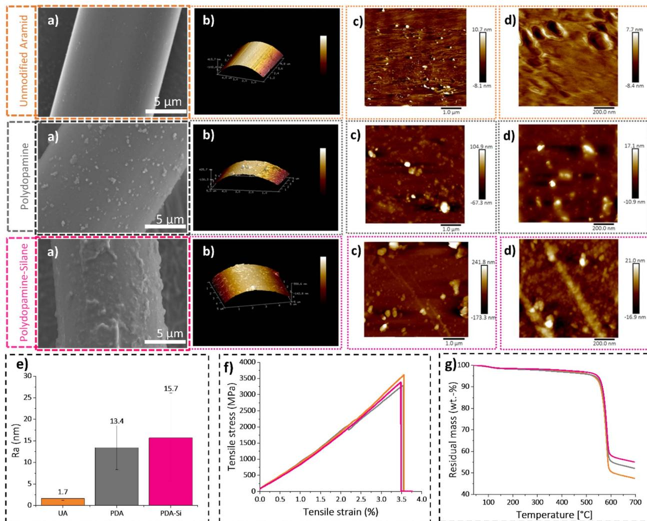
Fig. 4 (a) SEM images of the fiber surface, (b) AFM 3D view of the fiber surface with a scan size of  $5\ \mu\text{m} \times 5\ \mu\text{m}$ , (c) 2D view of the fiber topography with a scan size of  $5\ \mu\text{m} \times 5\ \mu\text{m}$ , (d) 2D view of the fiber topography with a scan size of  $1\ \mu\text{m} \times 1\ \mu\text{m}$ , and (e) calculated roughness parameters. (f) Mechanical properties and (g) thermogravimetric analysis of UA (orange), PDA (grey) and PDA Si (pink).
