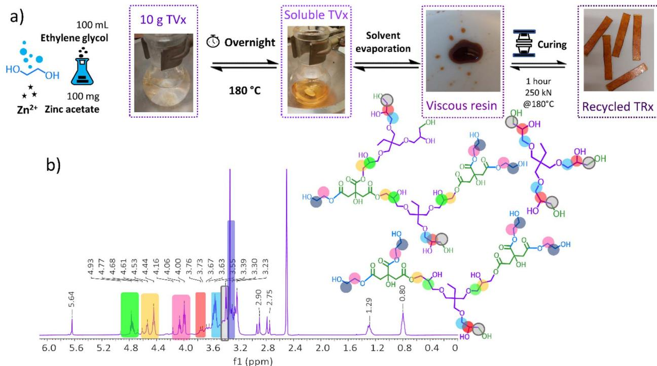
Fig. 7 (a) Chemical recycling methodology through transesterification exchange reactions. (b) Spectroscopic characterization of the viscous resin performed in deuterated DMSO by <sup>1</sup>H NMR.
